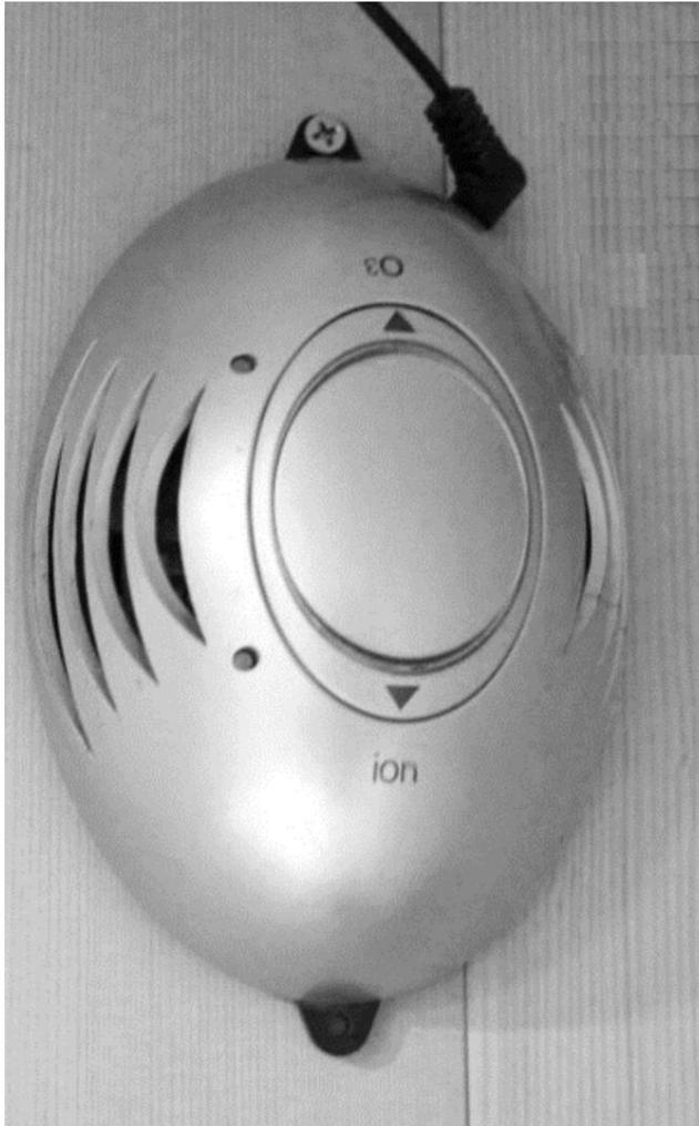
The ION button is used to switch on the ionizer. After pressing, the control diode lights up - green.
